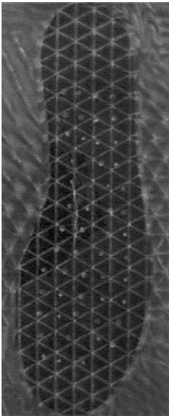
**Fig 1.** Magnetic field visualization with superimposed magne-view film. The microencapsulated colloidal nickel particles congregate in alignment with the magnetic flux lines producing a 2-dimensional image of the pole pattern.
